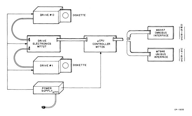
Figure 1-1 Floppy Disk System Configuration
