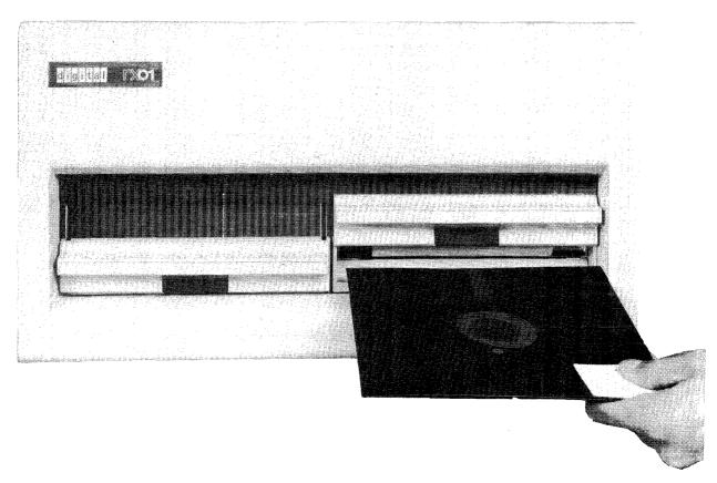
Figure 2-7 Flexible Diskette Insertion
