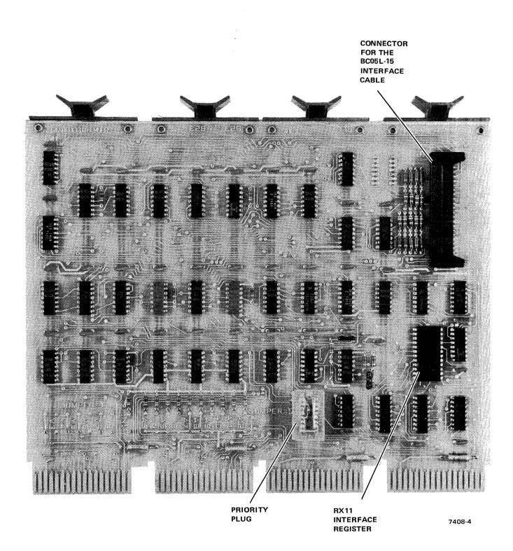
Figure 1-4 M7846 Module (RX11 Interface)
