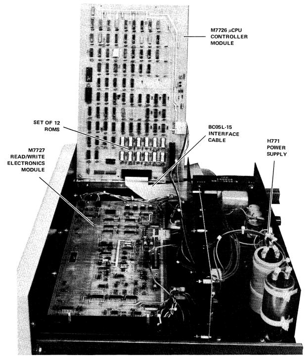
Figure 1-5 Top View of the RX01
