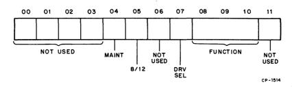
Figure 4-2 Command Register Format (RX8E)
