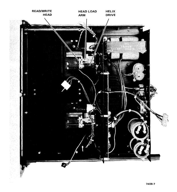
Figure 1-7 Top View of Drive
