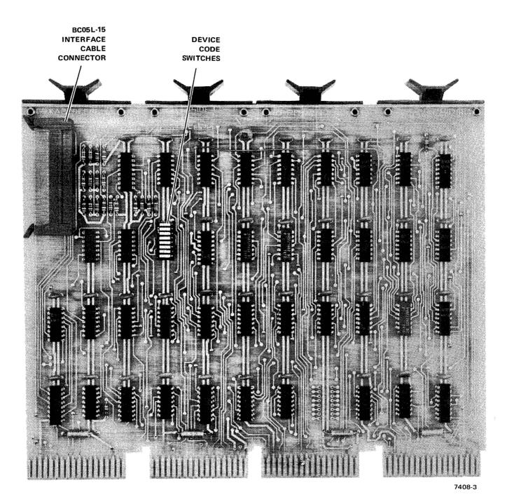
Figure 1-3 M8357 Module (RX8E Interface)
